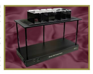
Each IITC Mesh stands are supplied with 5, 16" long, black anodized posts, (16" posts eliminate laboratory technicians from having to strain when trying to view correct placement of EVF probes.), black anodized base. Mesh - black anodized with 1/4" size waffle holes and a clear Plexiglas animal enclosure which is placed on top of mesh; allowing unobstructed view of the animal subjects during testing.
